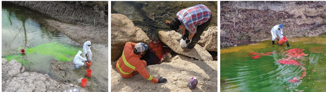
Figure 3- Dye injection photos: (left) Howard Ranch Swallet; (middle) Bigote Swallet; (right) South Onion Creek at Gatlin Creek Rd. crossing.
